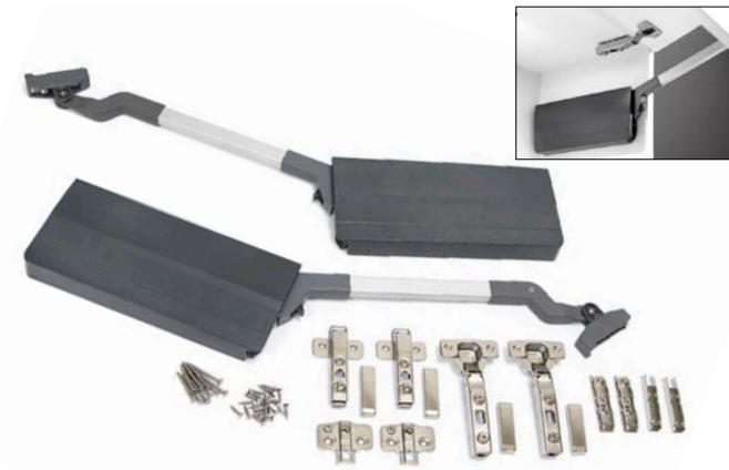
AGILE Flap Kit - For Door heights 650 - 729mm (Max. Door Width 1800mm) 40VA upto 7.2kg 41VA over 7.2kg
